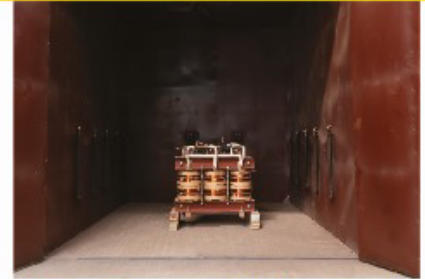
Transformer Heat Chamber
