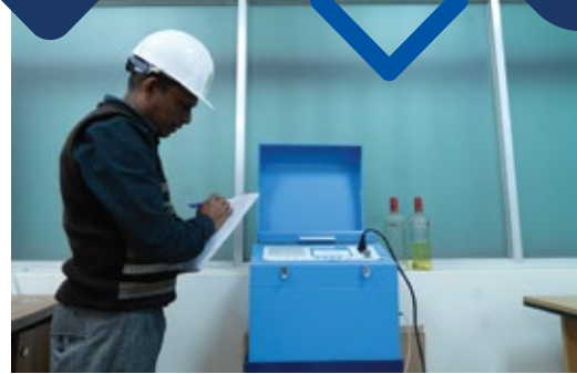
Transformer Oil Test
