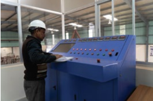
Transformer Test Bench
